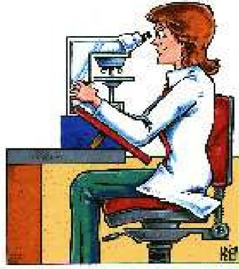
**AFTER** : Height-adjustable the microscope allows comfortable, upright work posture
